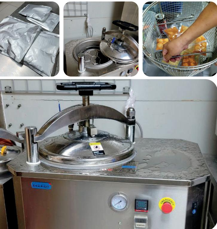
Retort machines sterilizes food products in sealed containers, such as cans or jars, to extend their shelf life. It uses heat to eliminate harmful microorganisms and can be designed to handle different types of food products. The FAF retort machine, that is sponsored by KPDNHEP, allows us to repack ready-to-eat meals so that food shelf life can be extended.
